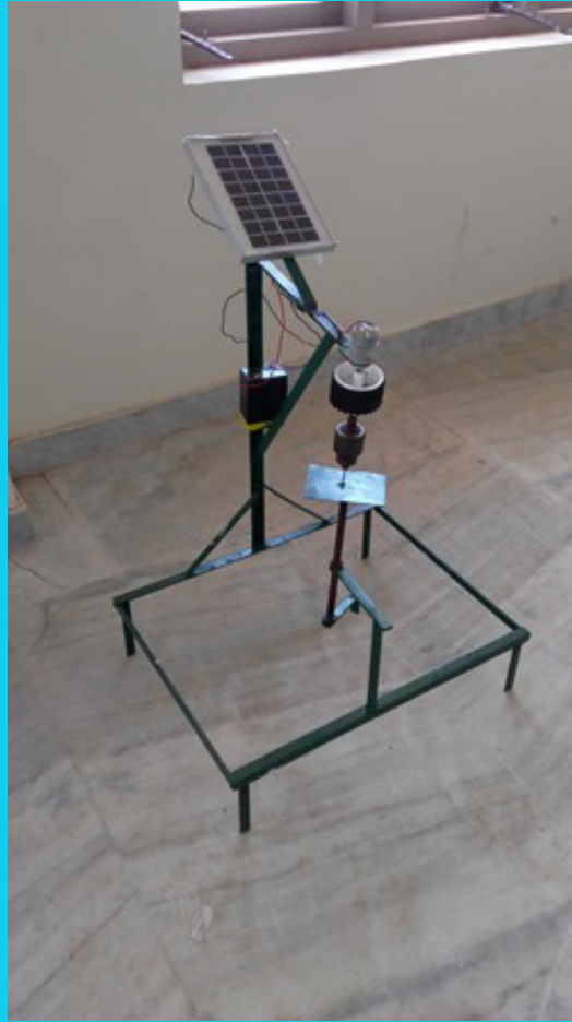
5. Solar power drilling machine
